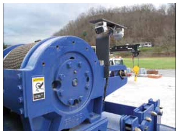
Cameras display the winch as well as the blind area directly behind the crane. Full color video display in operator cab is standard equipment.
