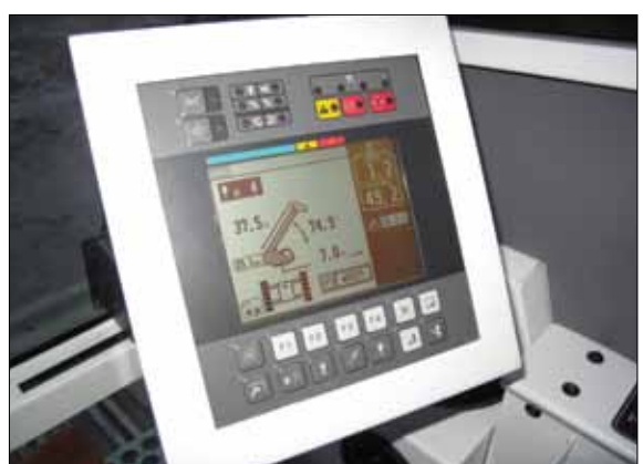
Tadano AML-C rated capacity indicator provides continuous feedback of crane lift position and data
